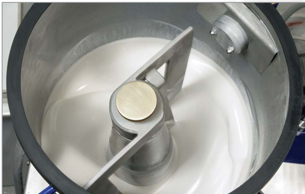
Mixing action of Maxivac 17 mixer.
