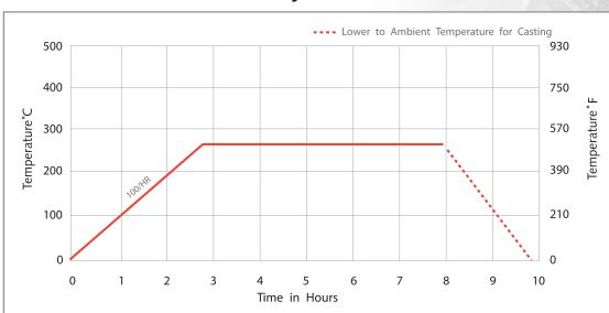
Note: Do not remove flasks from furnace to cast until they have been held at casting temperature for a minimum of 1 hour. If held for less than 1 hour, the core of the flasks will be at a much higher temperature than the digital temperature display states, and may result in metal mould reaction.
