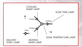
The controller ramps the burnout furnace at the specified rate until the required soak temperature is reached. The program then controls the furnace temperature at the specified soak temperature for the desired length of time. Once this step is complete the controller then runs through the subsequent steps until the program is complete. Once the program is complete the controller will display "END".
